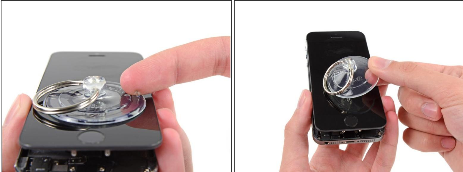
**⚠** Do not try to completely remove the front panel assembly from the rear case, as there are several delicate ribbon cables connecting them.
