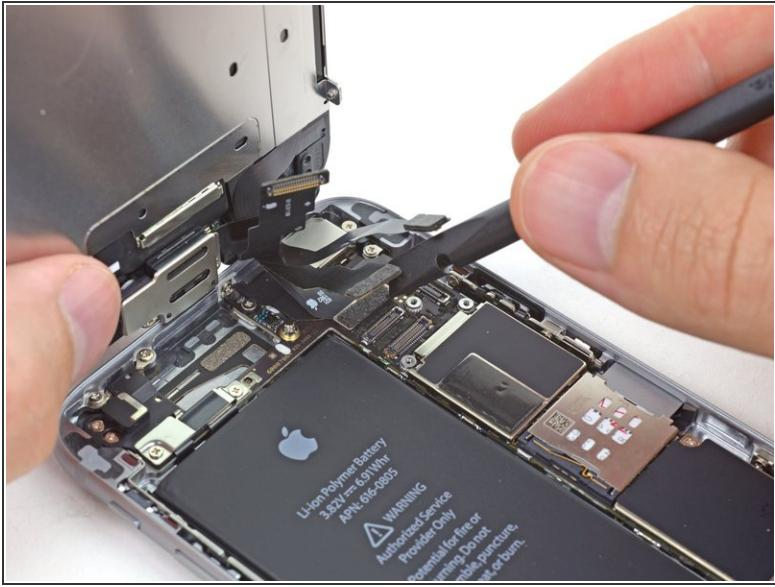
! Make sure the battery is disconnected before you disconnect or reconnect the cable in this step.
