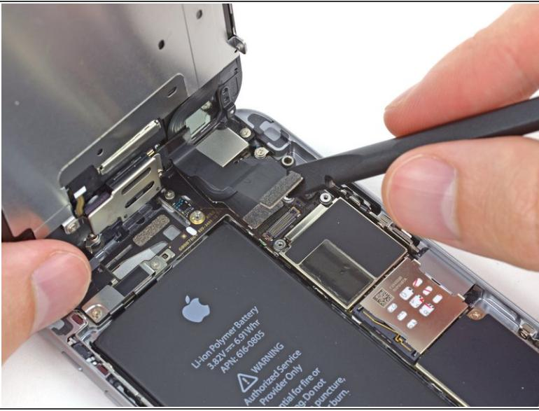
**⚠** In the next four steps, take care to pry up **only** on the cable connectors, and not on their sockets on the logic board.
