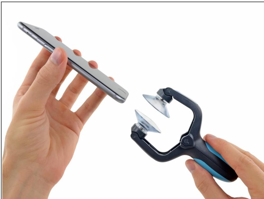
**i** The next three steps demonstrate using the iSclack, a great tool for safely opening the iPhone 6 that we recommend for anyone doing more than one repair. **If you aren't using the iSclack, skip down three steps for an alternate method.**
