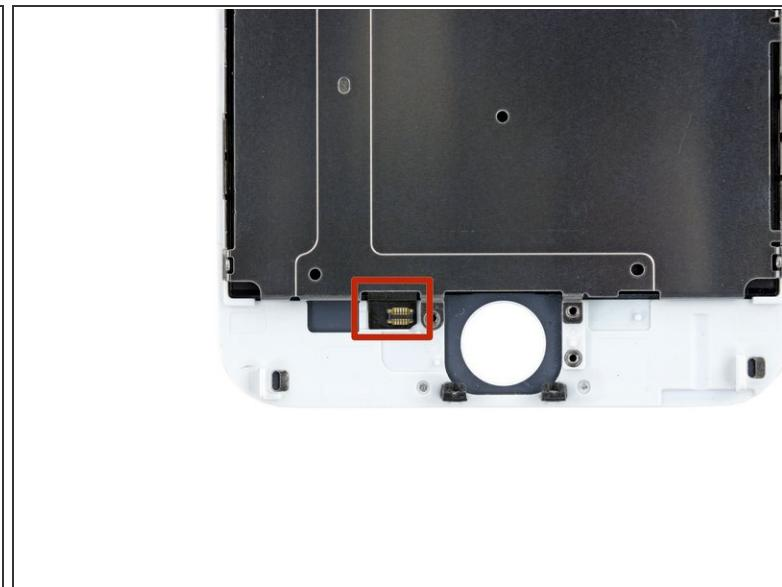
*(i)* The next step requires peeling one end of the home button cable (highlighted in red in the second picture) that is affixed to the back of the display assembly with strong adhesive. We highly recommend [using an iOpener](#) to heat the bottom of the display assembly, directly on top of the home button.
