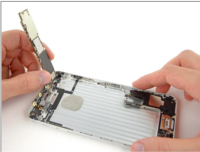
**⚠ Do not remove the logic board. At this point it is still tethered to the rear case via an antenna connector.**
