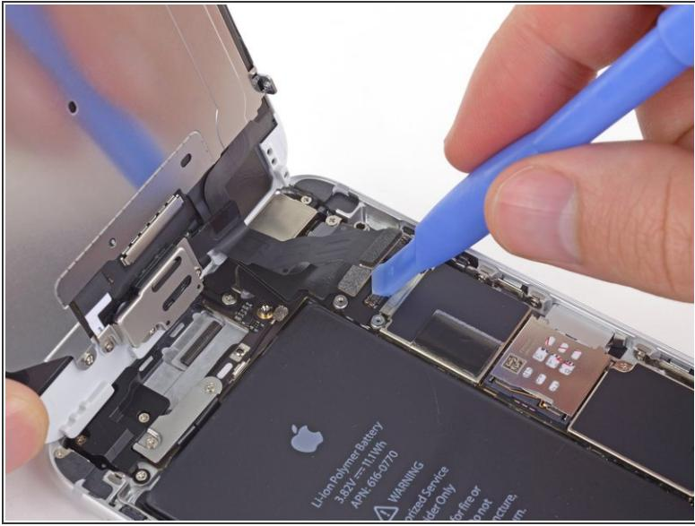
⚠ In the next four steps, take care to pry up **only** on the cable connectors, and not on their sockets on the logic board.
