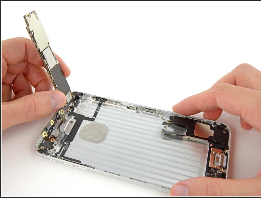
**⚠** Do **not** remove the logic board. At this point it is still tethered to the rear case via an antenna connector.
