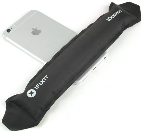
**i** The next step requires peeling up the Lightning connector and headphone jack cable that is affixed to the inside of the rear case with mild adhesive. We highly recommend [using an iOpener](#) on the lower backside of the rear case to soften the adhesive.
