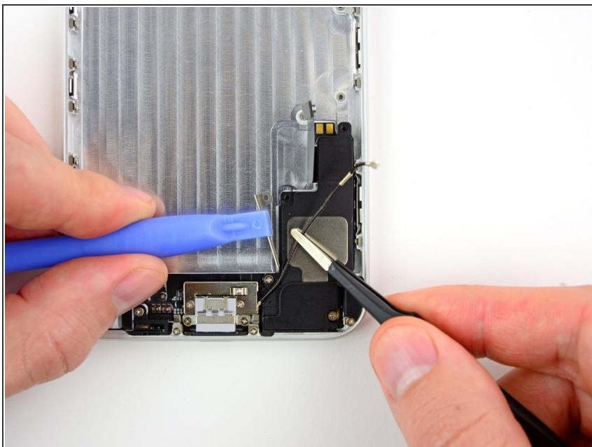
*i* To fully de-route the antenna connector, you may need to gently pull back the metal clip securing it to the speaker assembly.
