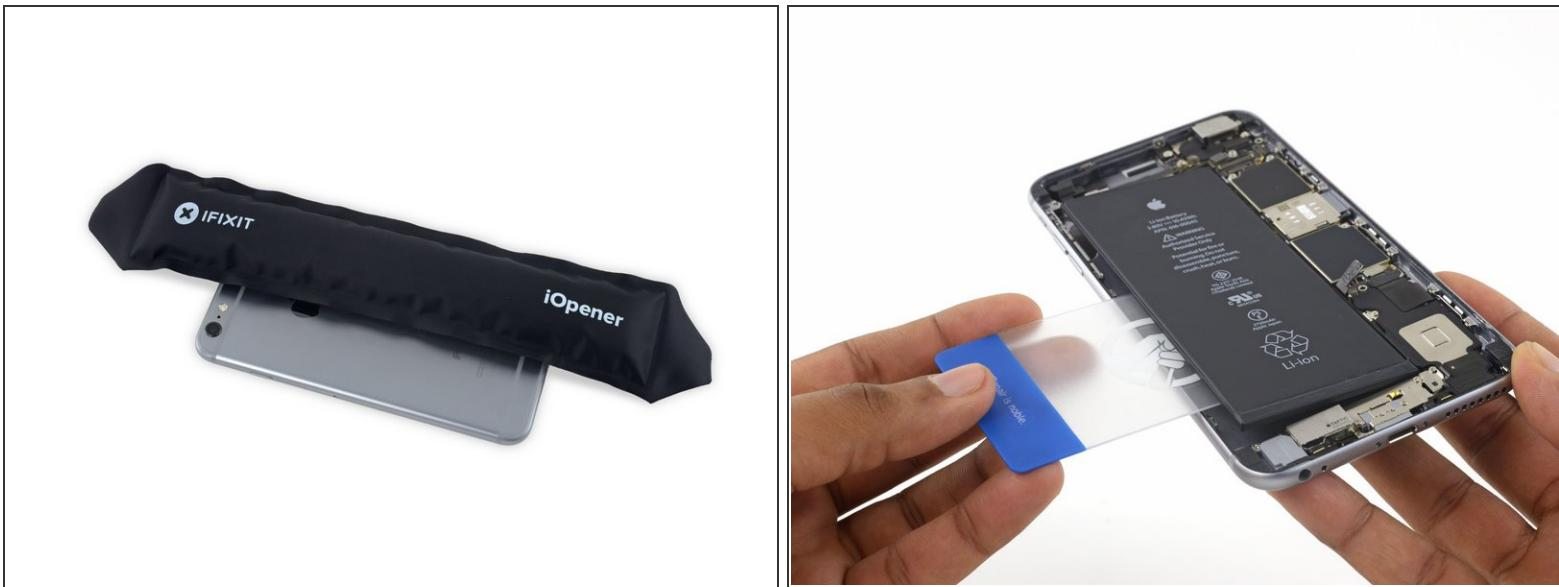
***(i)* If you successfully removed all three adhesive strips, move on to the next step.** Otherwise, you will need to pry the battery from the rear case.
