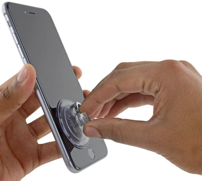
**i** Opening the display on the 6s Plus separates a thin strip of adhesive around the perimeter of the display. If you prefer to replace the adhesive, have a set of new adhesive strips ready before you continue. It's possible to complete the repair without replacing the adhesive, and you probably won't notice any difference in functionality.
