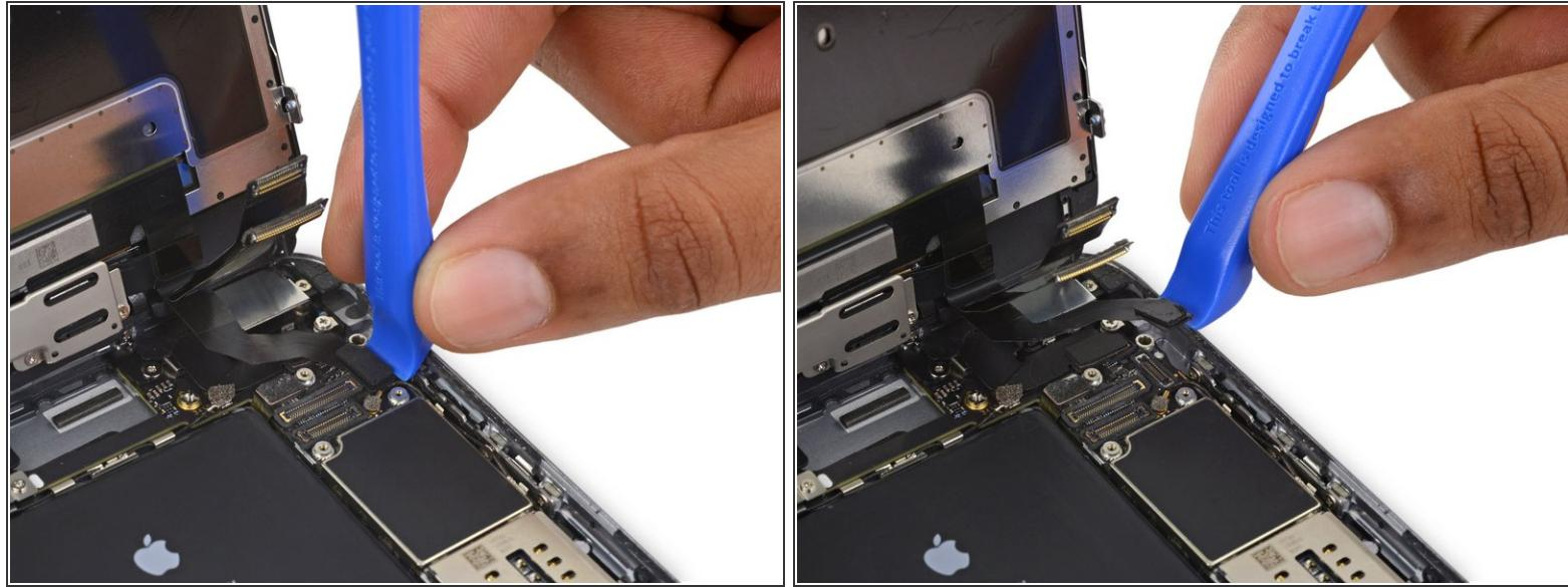
⚠ Make sure the battery is disconnected before you disconnect or reconnect the cable in this step.
