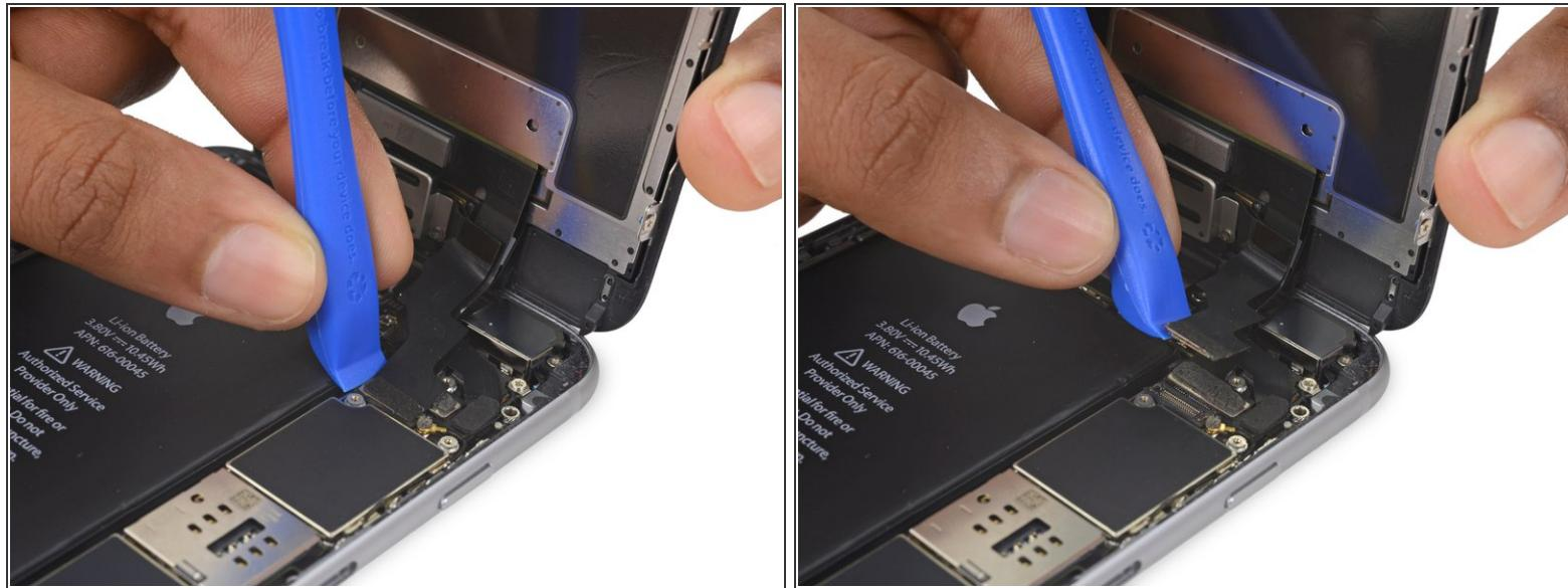
**⚠** Be careful to only pry up on the connector itself and not the socket on the logic board.
