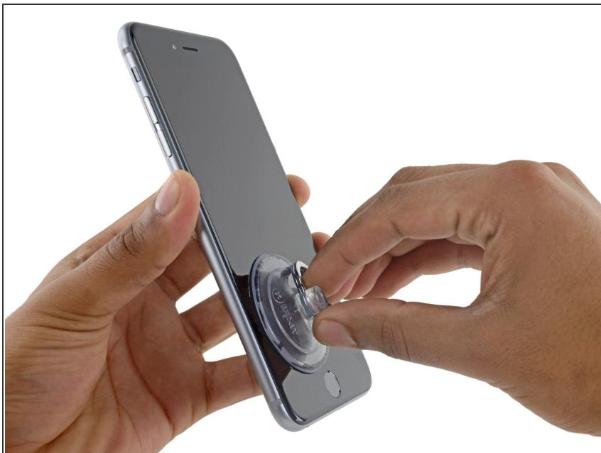
**i** Opening the display on the 6s Plus separates a thin strip of adhesive around the perimeter of the display. If you prefer to replace the adhesive, have a set of new adhesive strips ready before you continue. It's possible to complete the repair without replacing the adhesive, and you probably won't notice any difference in functionality.
