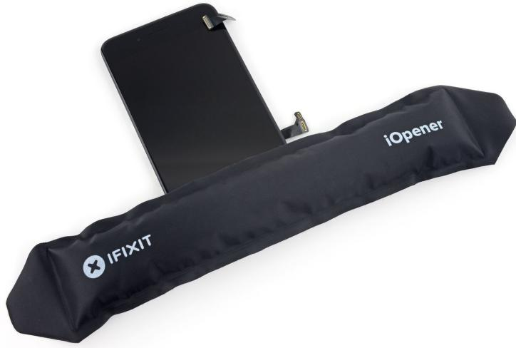
ⓘ Heating the area around the home/Touch ID sensor will help soften the adhesive holding its delicate cable in place, making it easier to remove safely.
