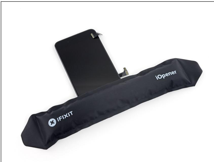
ⓘ Heating the area around the home/Touch ID sensor will help soften the adhesive holding its delicate cable in place, making it easier to remove safely.
