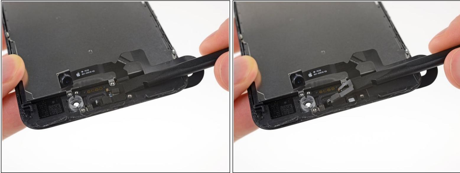
**⚠** The sensors on this step are fragile. To increase your chances of removing them without damage, use your iOpener or hair dryer to apply heat to the upper portion of the display before you proceed. Alternatively, add a drop or two of isopropyl alcohol and let it penetrate under the sensors before you pry them up.
