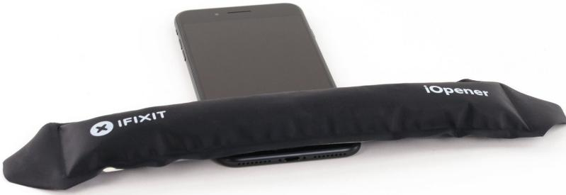
**i** Heating the lower edge of the iPhone will help soften the adhesive securing the display, making it easier to open.
