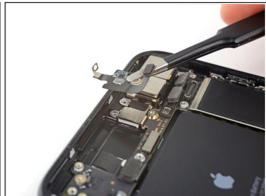
*(i)* The screw boss at the top of the antenna flex cable is tucked into a small recess in the top edge of the iPhone.
