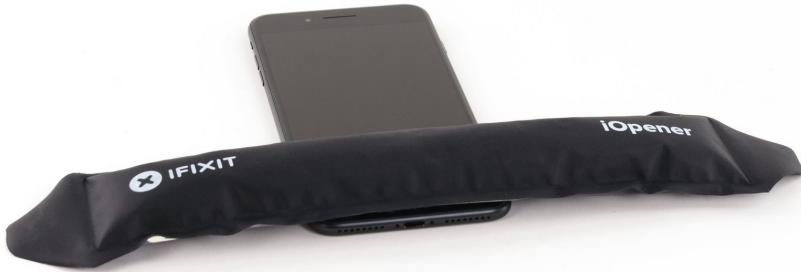
**i** Heating the lower edge of the iPhone will help soften the adhesive securing the display, making it easier to open.
