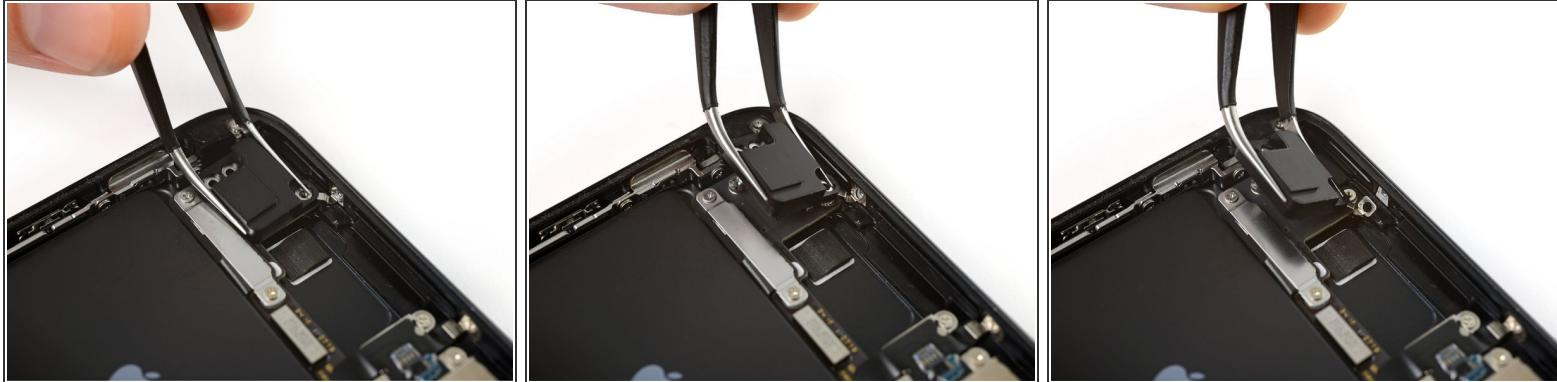
*(i)* The screw boss at the top of the antenna component is tucked into a small recess in the top edge of the iPhone.
