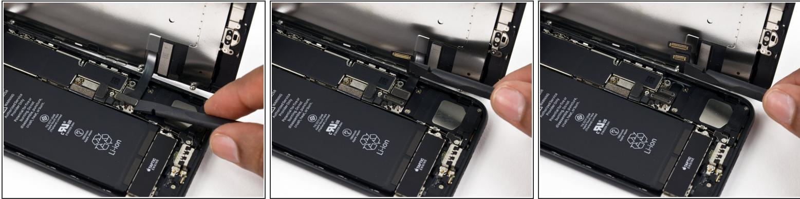
**⚠** Make sure the battery is disconnected before you disconnect or reconnect the cables in this step.
