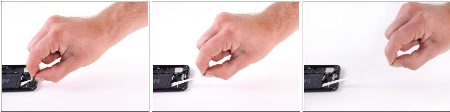
**⚠** Try to keep the strips flat and unwrinkled during this procedure; wrinkled strips will stick together and break instead of pulling out cleanly.
