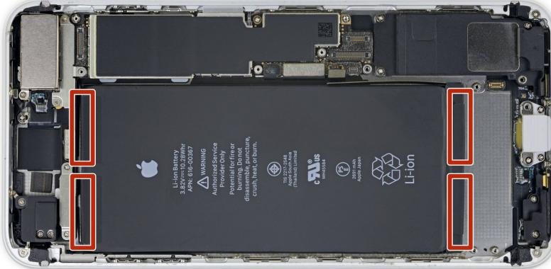
**i** The iPhone 8 Plus's battery is secured by four pieces of stretch-release adhesive—two at the top, and two at the bottom.
