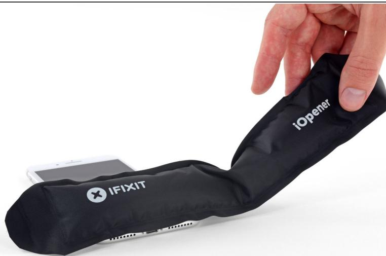
**i** Heating the lower edge of the iPhone will help soften the adhesive securing the display, making it easier to open.
