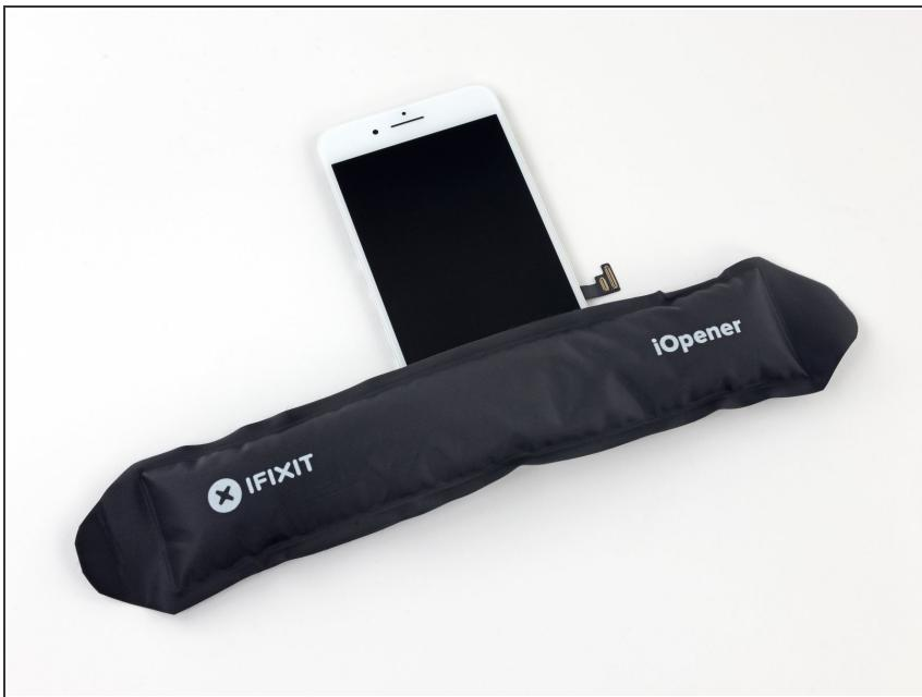
**i** Heating the area around the home/Touch ID sensor will help soften the adhesive holding its delicate cable in place, making it easier to remove safely.
