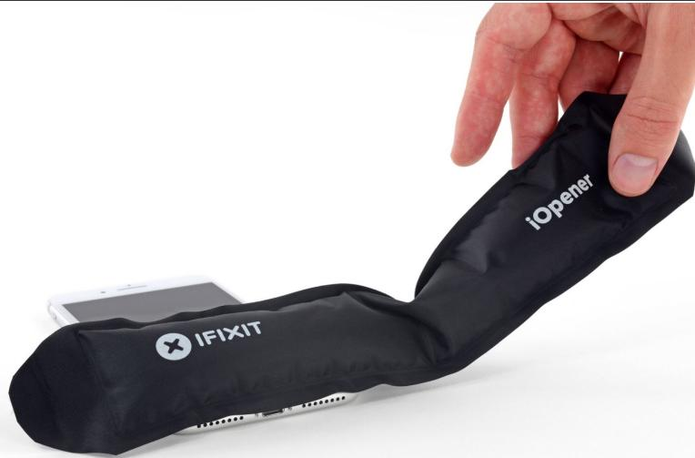
ⓘ Heating the lower edge of the iPhone will help soften the adhesive securing the display, making it easier to open.
