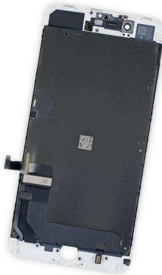
Compare your new replacement part to the original part—you may need to transfer remaining components or remove adhesive backings from the new part before installing.
