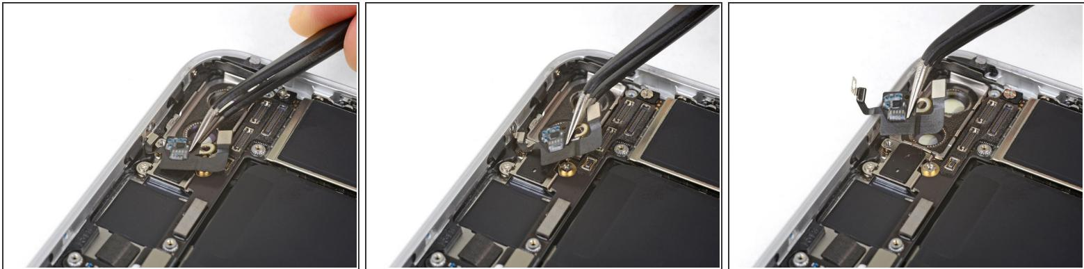
ⓘ The screw boss at the top of the antenna flex cable is tucked into a small recess in the top edge of the iPhone.
