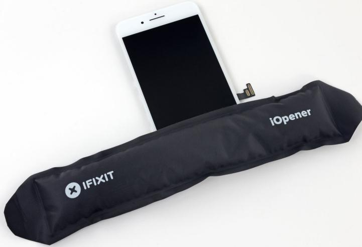
**i** Heating the area around the home/Touch ID sensor will help soften the adhesive holding its delicate cable in place, making it easier to remove safely.
