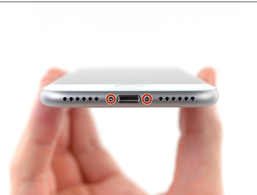
**⚠** Before you begin, discharge your iPhone battery below 25%. A charged lithium-ion battery can catch fire and/or explode if accidentally punctured.
