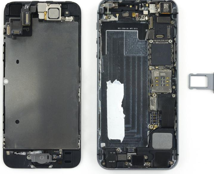
**i** If your phone was fully submerged for any amount of time, it is likely some of the internal components corroded. Corrosion looks like a white, chalky film covering metallic surfaces, and is especially prevalent on pins and connectors that carry current. Corrosion dissolves metals and will cause malfunctions in your phone.
