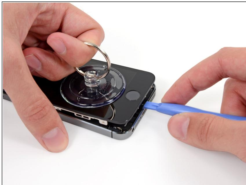
**⚠** The front panel is attached with clips, and there are several ribbon cables connecting it to the rest of the phone. Your goal here is to release the clips and **open the phone only enough to disconnect the cables**. Go slowly and carefully to avoid damage.
