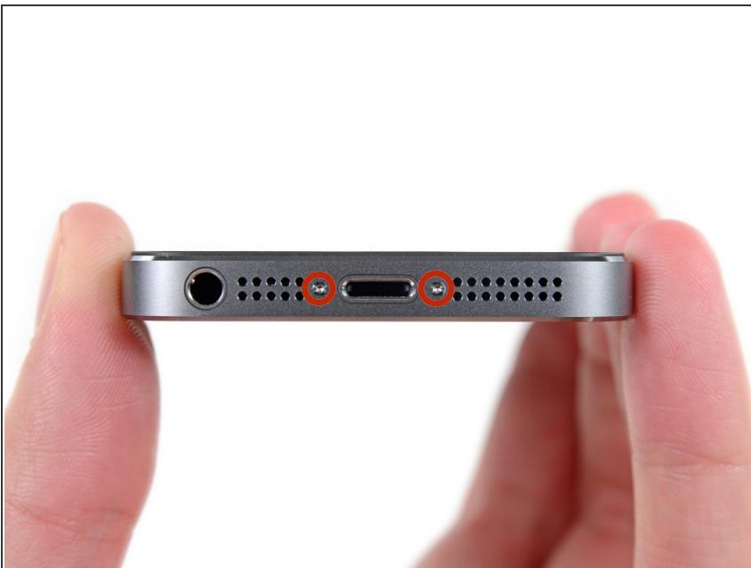
**⚠** Before you proceed, discharge your iPhone battery below 25%. A charged lithium-ion battery can catch fire and/or explode if accidentally punctured.
