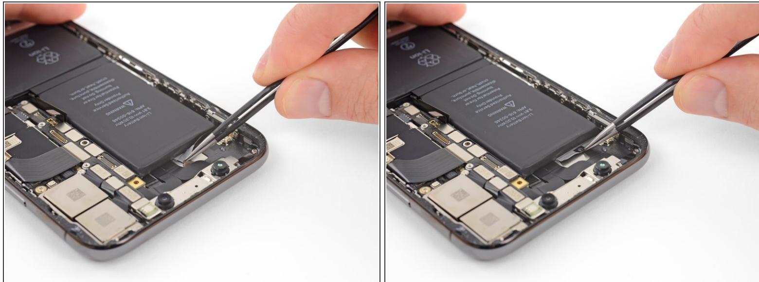
⚠ The final pull tab lies very close to the Face ID hardware. If damaged, Face ID can only be repaired by Apple, so work with care.
