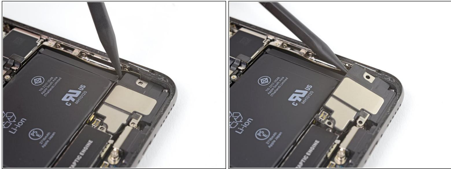
**⚠** When prying up the speaker, take care not to damage the flex cable you just disconnected. If necessary, hold it to one side so the speaker has room to come out.
