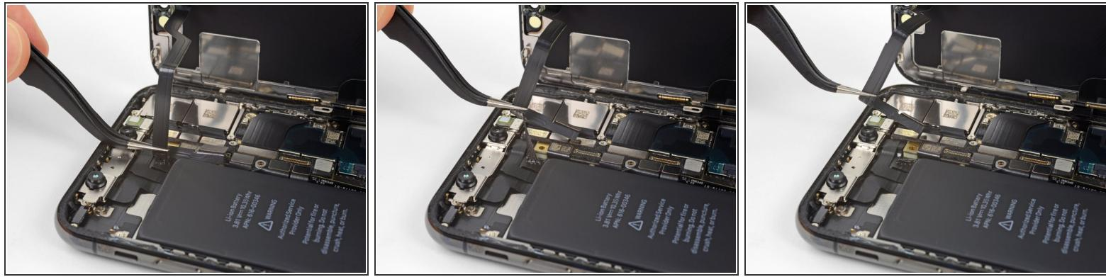
**i** The front panel sensor assembly flex cable is lightly adhered in place.
