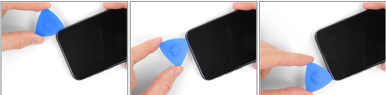
i The top edge of the display is secured with both glue and clips.
