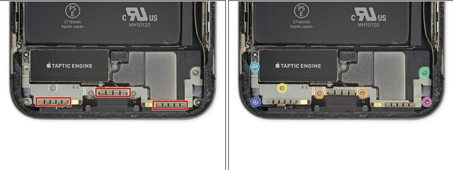
⚠ Be careful not to touch the three rows of grounding pads near the bottom of the iPhone.
