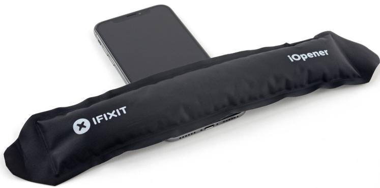
ⓘ Heating the lower edge of the iPhone will help soften the adhesive securing the display, making it easier to open.
