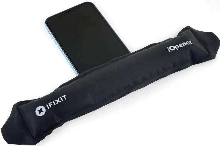
**i** Heating the lower edge of the iPhone helps soften the adhesive securing the display, making it easier to open.
