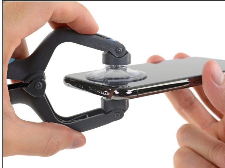
*(i)* The next two steps demonstrate the iSclack, a handy tool that we recommend for anyone doing frequent repairs. **If you aren't using the iSclack, skip down two steps for an alternate method.**
