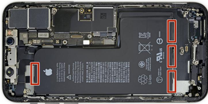
*(i)* The battery is secured to the rear case by four pieces of stretch-release adhesive—one under the upper area of the battery, and three under the lower area.
