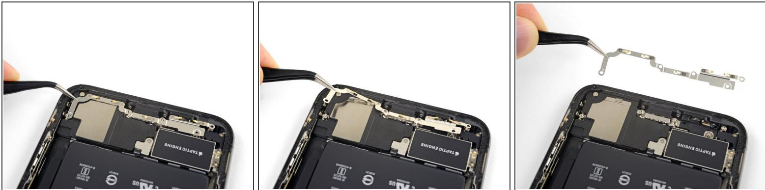
*(i)* The bracket is lightly adhered in place.
