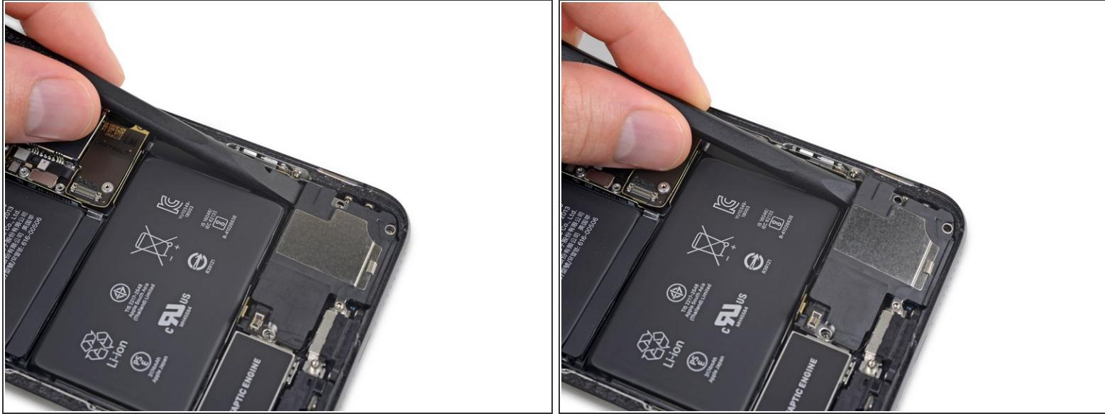
**⚠** When prying up the speaker, take care not to damage the speaker flex cable you just disconnected. If necessary, bend the cable toward the battery so the speaker has room to come out.
