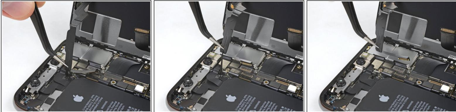
ⓘ The front panel sensor assembly flex cable is lightly adhered in place.
