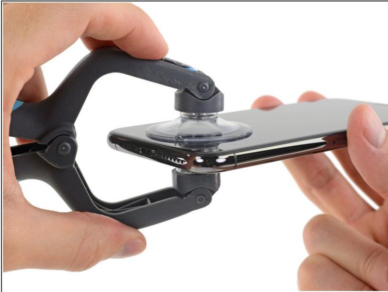
*(i)* The next two steps demonstrate the iSlack, a handy tool that we recommend for anyone doing frequent repairs. **If you aren't using the iSlack, skip down two steps for an alternate method.**
