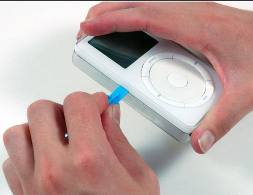
**i** Opening the iPod can be challenging. Don't get discouraged if it takes a few tries before the iPod is opened.
