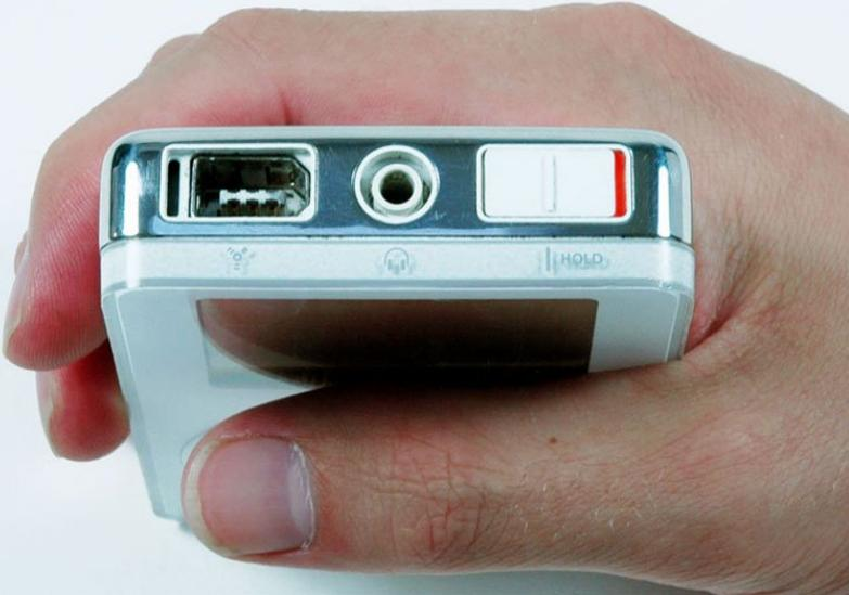
**i** Before opening your iPod, ensure that the hold switch is in the locked position.
