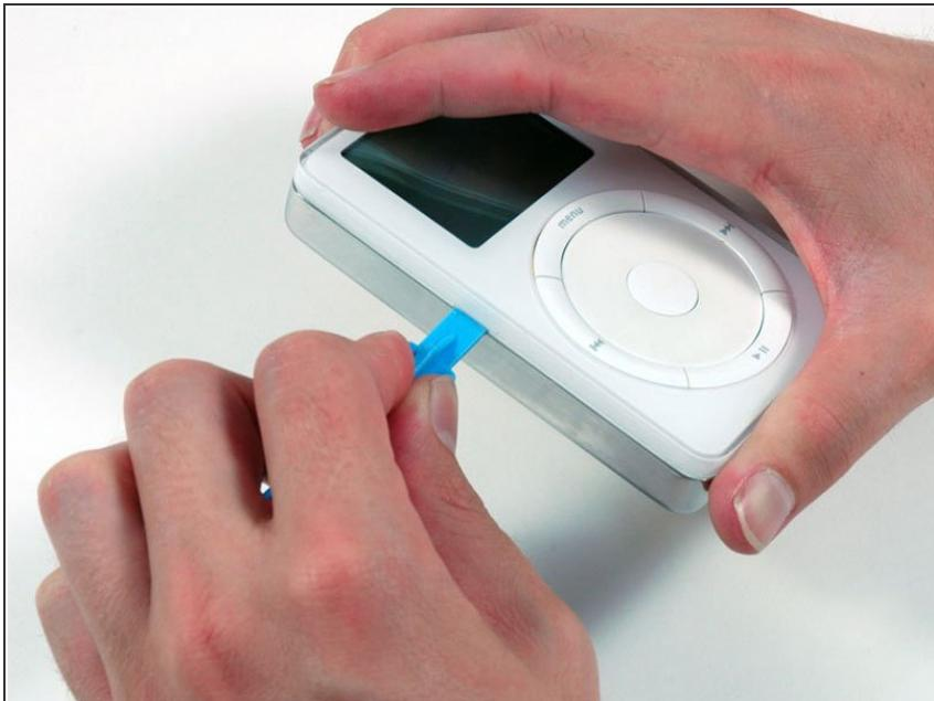
**i** Opening the iPod can be challenging. Don't get discouraged if it takes a few tries before the iPod is opened.
