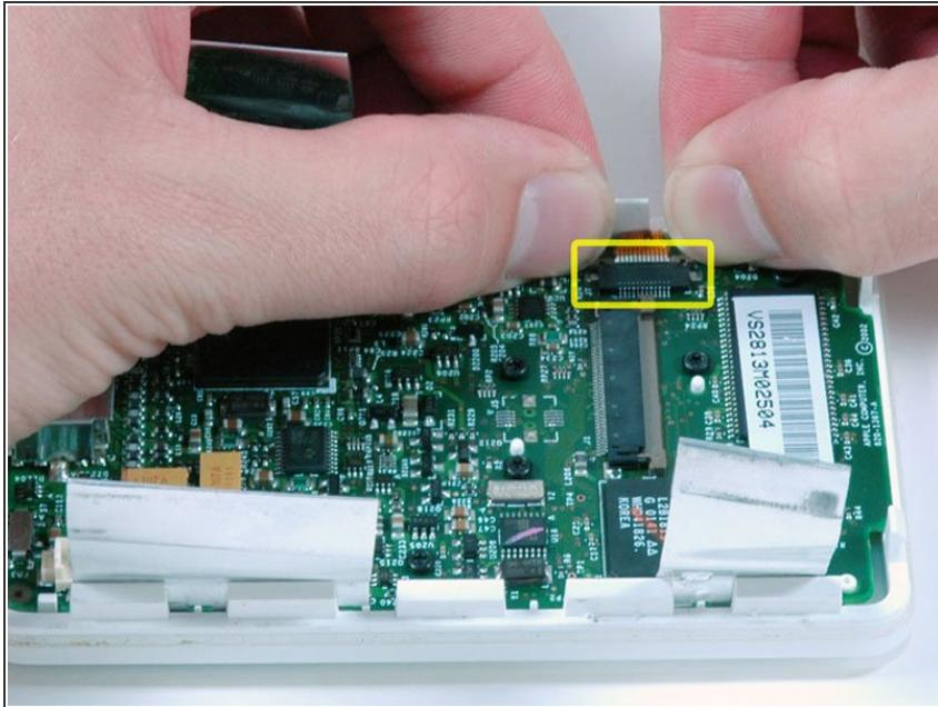
ⓘ Like the hard drive connector, for the following step, you only need to move the connector about 2 mm. Pushing too hard or too far will damage the connector.
