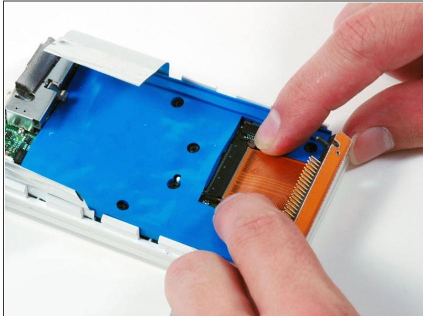
*(i)* For the following step, you only need to move the locking bar about 2 mm. Pushing too hard or too far will damage the connector.
