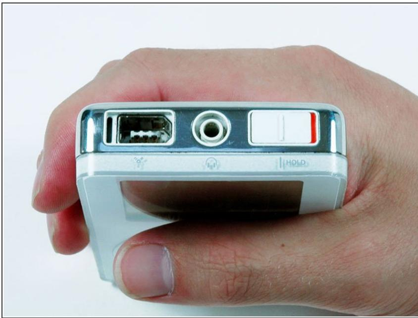
**i** Before opening your iPod, ensure that the hold switch is in the locked position.
