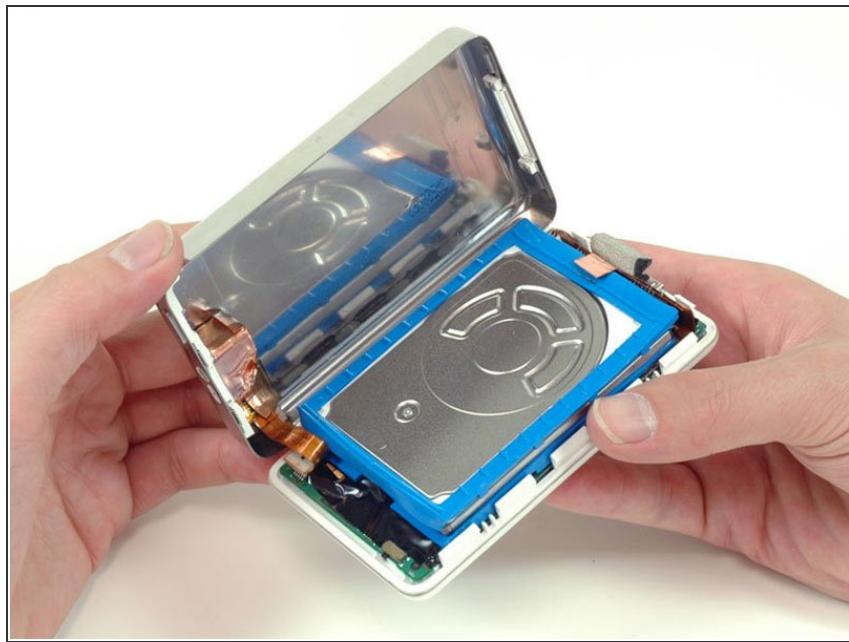
**i** The iPod case is now open, but don't separate the two halves just yet. There is still an orange ribbon cable connecting the headphone jack to the logic board.
