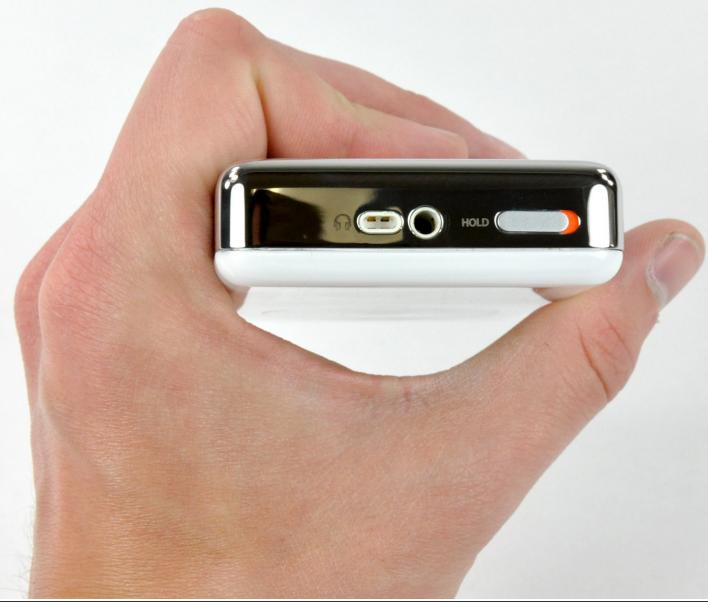
ⓘ Before opening your iPod, ensure that the hold switch is in the locked position. The orange bar should be visible, indicating hold is active.
