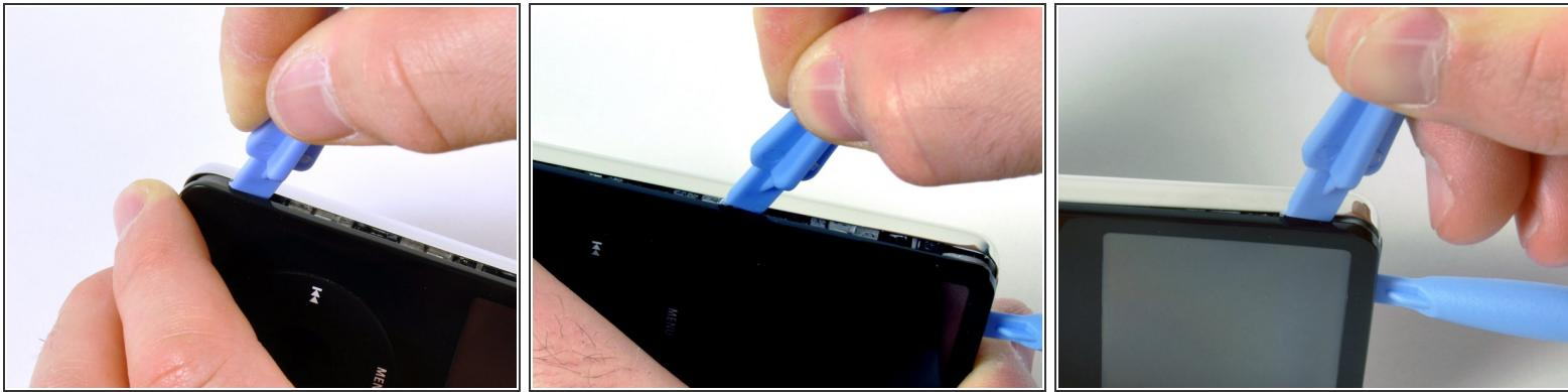
ⓘ There are four retaining clips on each side of the iPod. An iPod opening tool will be used to separate the plastic front from the metal back of the iPod.
