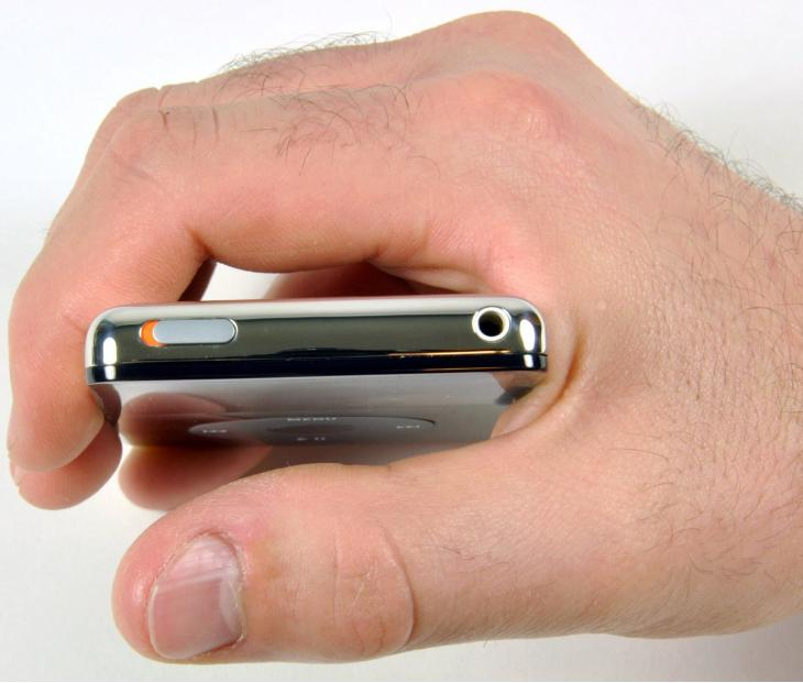
**i** Before opening your iPod, ensure that the hold switch is in the locked position. The slider should be all the way to the right if your iPod is facing you.
