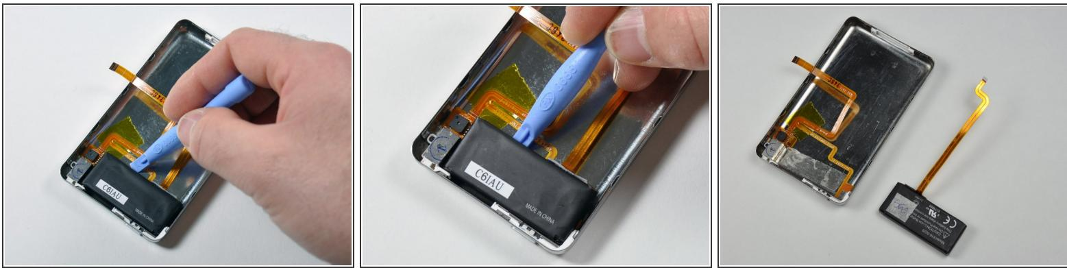
! Be careful not to damage any of the headphone or battery ribbon cables while performing this step.
