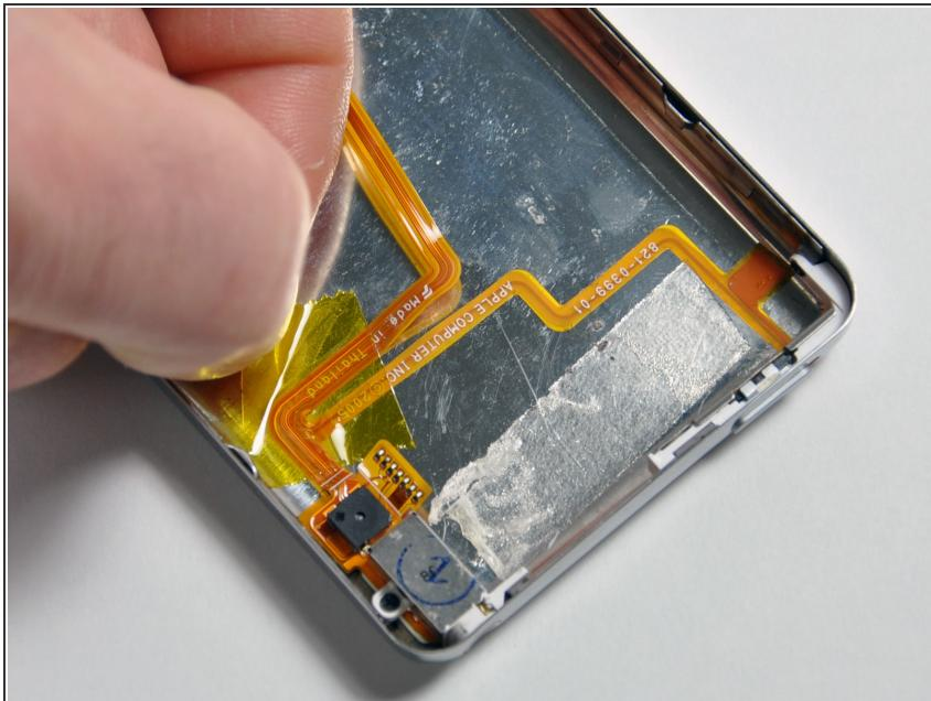
! Be very careful when performing this step, since the orange ribbon cables can easily be broken.
