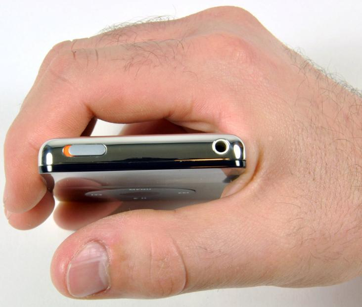
ⓘ Before opening your iPod, ensure that the hold switch is in the locked position. The slider should be all the way to the right if your iPod is facing you.
