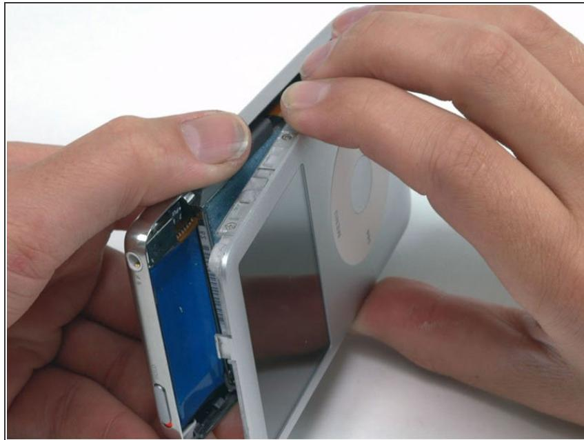
**⚠** There are two ribbon cables connecting the rear panel to the rest of the iPod. In the following step, be careful not to damage these ribbon cables.
