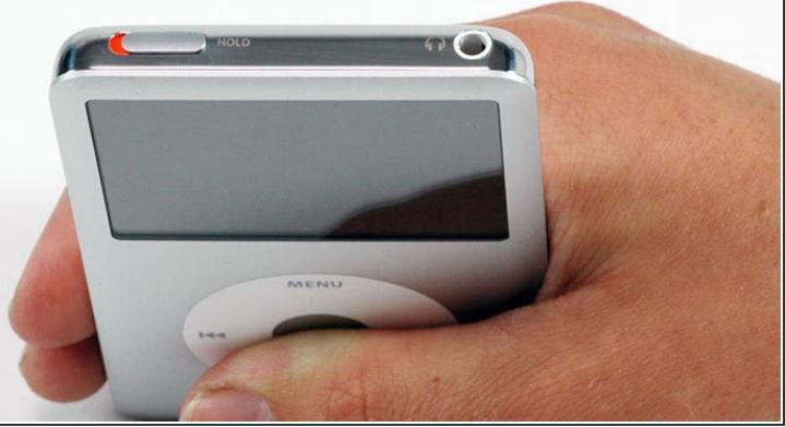
ⓘ Apple designed their new iPods to be very difficult to take apart without destroying major components. Because of the metal faceplate, the metal backing, and the 13 (yes, 13) metal clips holding the case together, this is one of the toughest iPods to disassemble.
