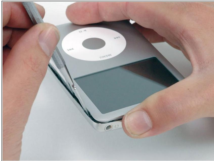
**i** The metal clips near the corners are notorious for tenaciously gripping the front panel. It is necessary to disengage these clips in order to open the iPod.
