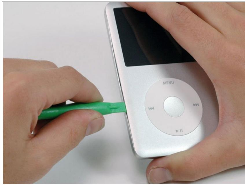
ⓘ Opening this iPod is challenging. Don't get discouraged if it takes you a few tries before the iPod is opened. One thing to notice is the angle of the plastic opening tool's tip while inserting it into the iPod. Ideally, the angle should be as vertical as possible while still clearing the edge of the rear panel.
