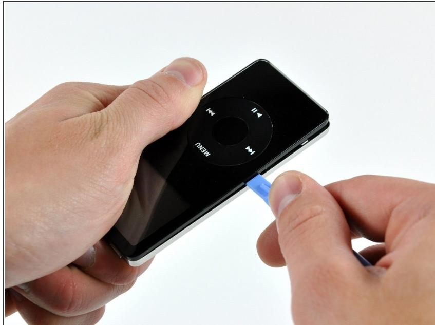
*(i)* The large iPod opening tool is no longer needed to gain access to the left side of the iPod.
